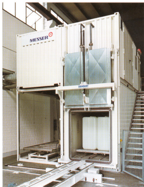
Fig. 5 Rail-mounted floor conveyor wagon for loading the fluorination plant (93.00.74.c)
