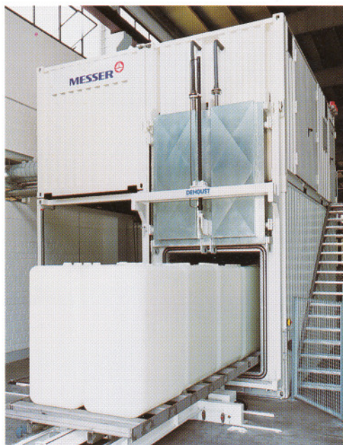
Fig. 4 Single vacuum chamber with 20 m 3 volume and two sealing doors (93.00.74.b)
