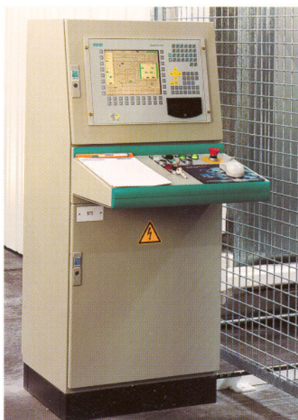
Fig. 6 Control console with process control computer (93.00.74.d)
